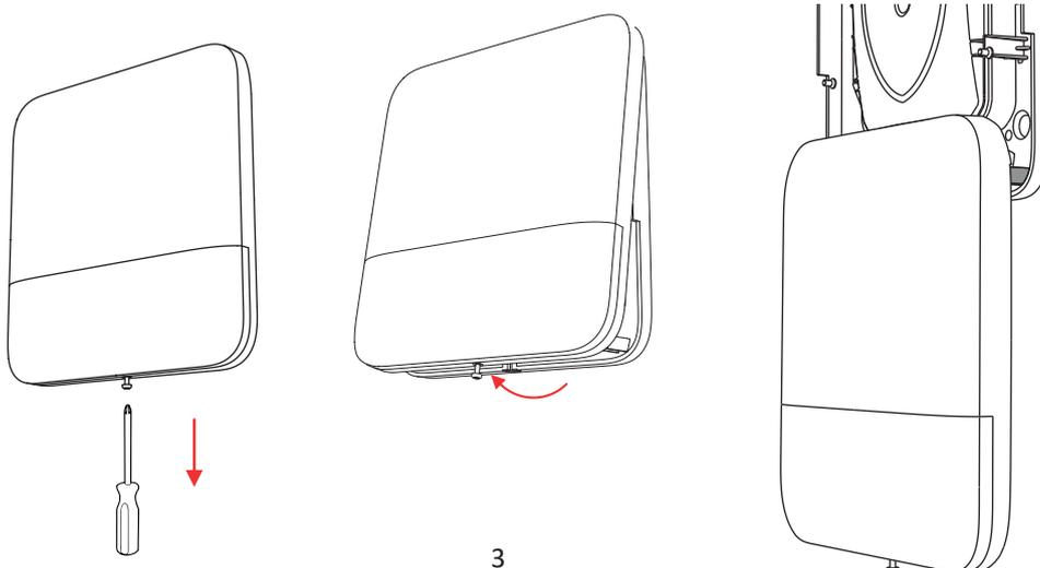
3. Attach the sounder to the required place with the top screw. Make the sounder horizontal by resorting to the gradienter.
