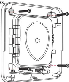
5. Fix the front panel on the sounder body. Tighten the set screw to complete the installation.
