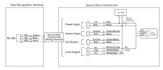
**Figure 4-6 Wiring Secure Door Control Unit**
