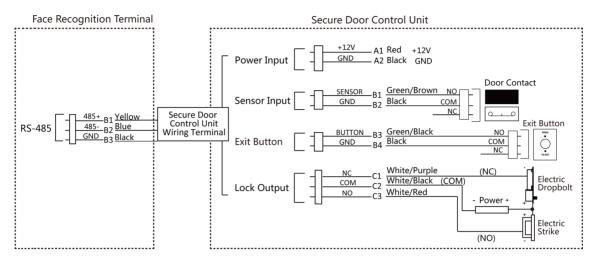
Figure 4-2 Secure Door Control Unit Wiring
