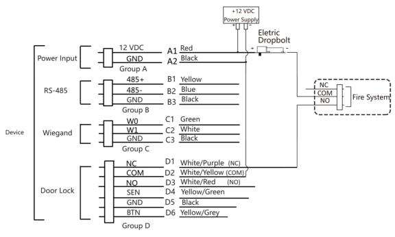
Figure 4-5 Wiring Device
