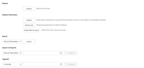
Note: The upgrading process will be 1 to 10 minutes, please don't disconnect power to the device during the process. The device reboots automatically after upgrading.
