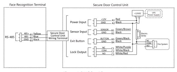
Figure 4-8 Wiring Diagram
