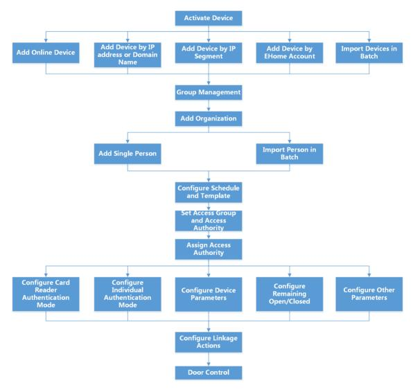
Figure 11-1 Flow Diagram of Configuration on Client Software
