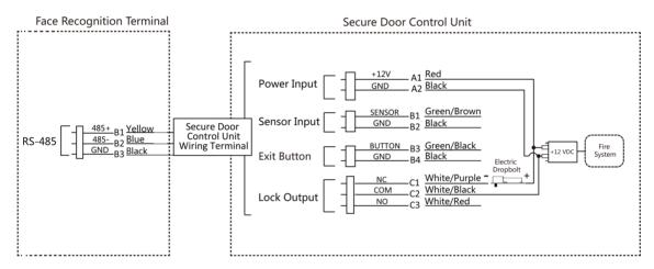
**Figure 4-4 Wire Secure Door Control Unit**
