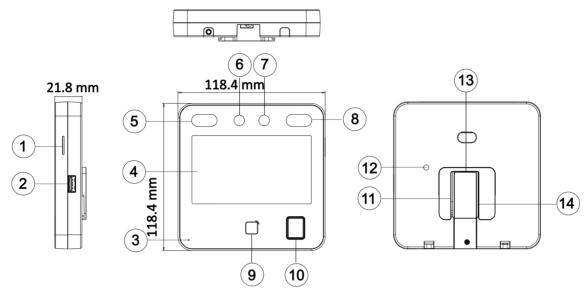
**Figure 2-1 Appearance (With Fingerprint)**
