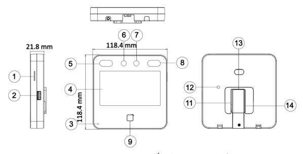
Figure 2-2 Appearance (Without Fingerprint)
