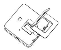
Figure 3-4 Place Bracket Close to Device Back Side
